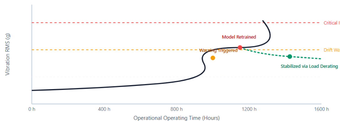
Figure 3: Real-Time Vibration RMS Degradation & Retraining Intervention Thresholds
